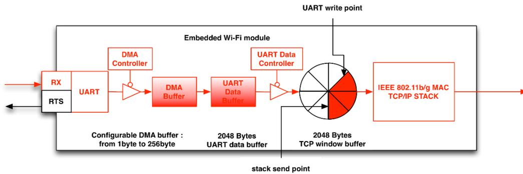
5. If network is blocked, it results in the TCP window Buffer filled with data, then no more data can be packed into TCP/IP package, it makes the DMA Buffer and UART Data Buffer also full of data. Under this situation, serial port cannot receive any more data that leads to the loss of data on serial port.
