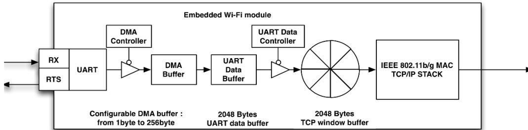
Firmware has three buffer used for temporary storage for serial data:
