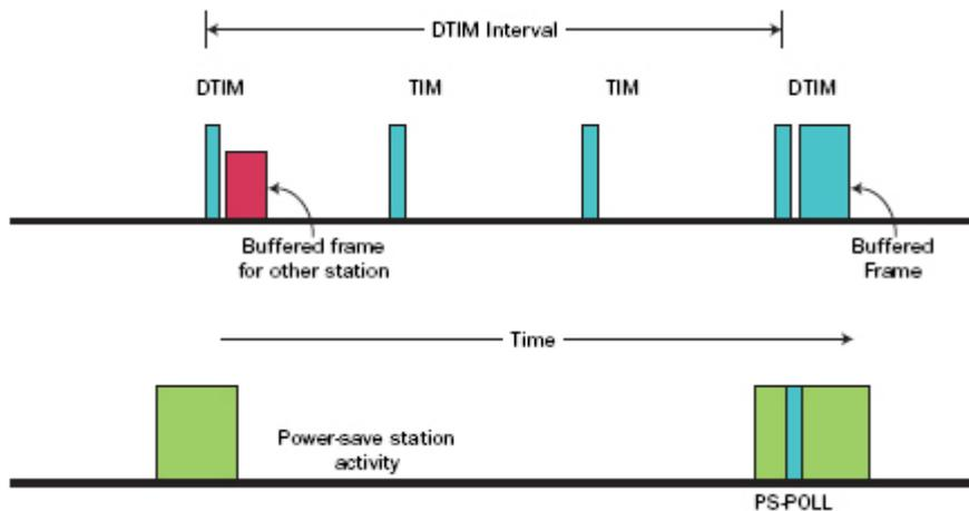
Every time module wakes up, it will check if AP has buffered data for module and receive them immediately. After has received them successfully, module will continue to sleep. But if more data is arrived when module is asleep, module can receive only at the next DTIM time point. Delay is generated in this situation.
