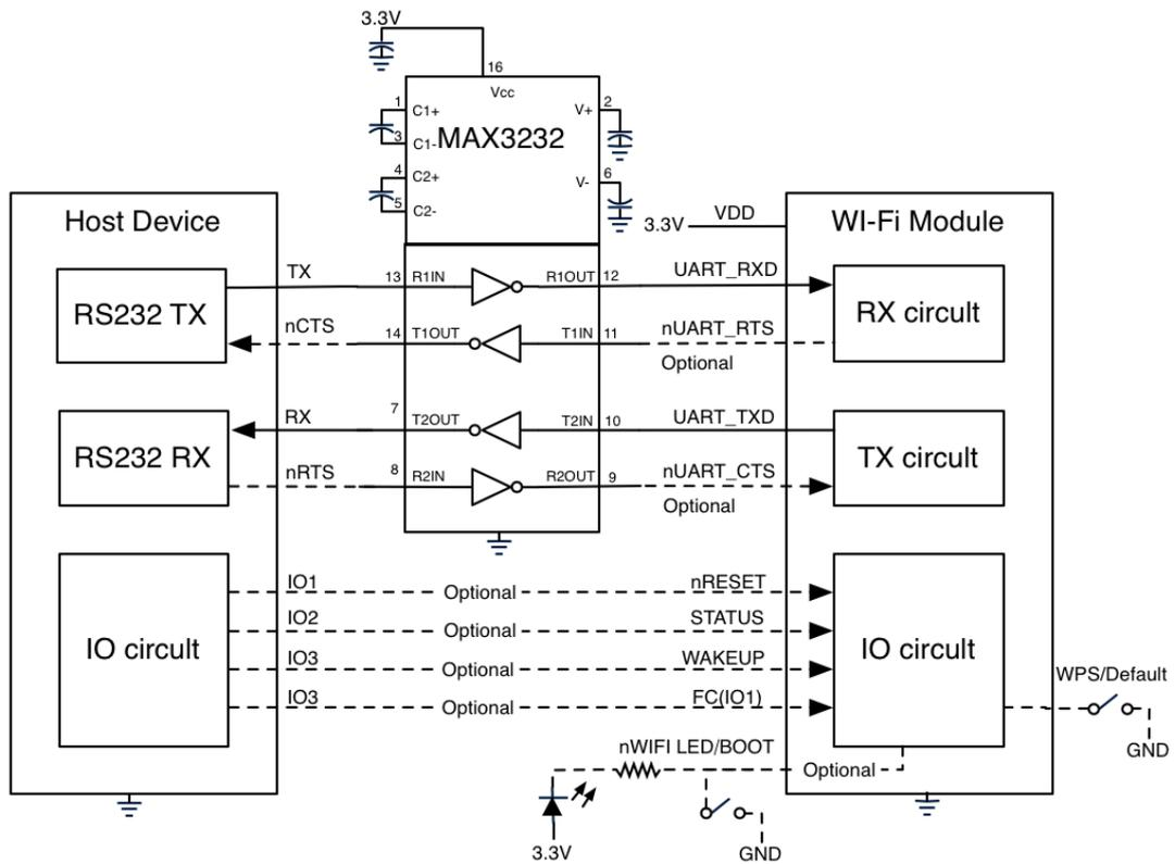
Figure 1.2 RS232 UART serial interface
