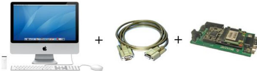
An USB-serial converter is available on EMW-380-S2 test board. It's very easy to connect the test board to PC via a mini USB cable. Set the jump J3, J4, J5, J6 to USB side and download the USB driver from <http://www.ftdichip.com/Drivers/VCP.htm>
