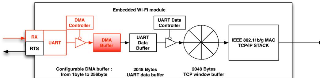
2. Firmware copy serial data from DMA buffer to UART data buffer when DMA buffer is full or timeout. DMA buffer size and timeout can be configured by *DMA buffer size* in order to balance the performance and delay. A larger size of DMA buffer size reduce the frequency of the copy operation and give more CPU time to processing network stacks that improve the system' s MAX of data
