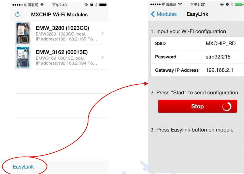
4. Wait the EasyLink negotiation complete, LED2 stop flashing and the module will reboot with the new settings. EasyLink negotiation timeout is 2 minutes. If EasyLink was failed, module would keep and use the old settings.
