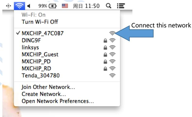
Once connected to the network, your pc would be assigned an IP address which within the scope of 192.168.1.XX. Now you can communicate with module, which has the static IP address: 192.168.1.1, and you can also locate module' s address by bonjour service. Login to module' s build-in web pages if you want to change module' s configuration, but we do not need to do this in this simple demonstration
