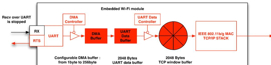
If *Hardware Flow Control* function is enabled, module would assert RTS signal under such situation to announce that sender should not send any more serial data. It can prevent the loss of data when network is blocked.
