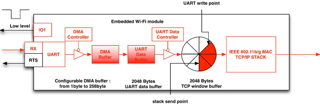
2. When the module sends out UART data, IO1 outputs high.
